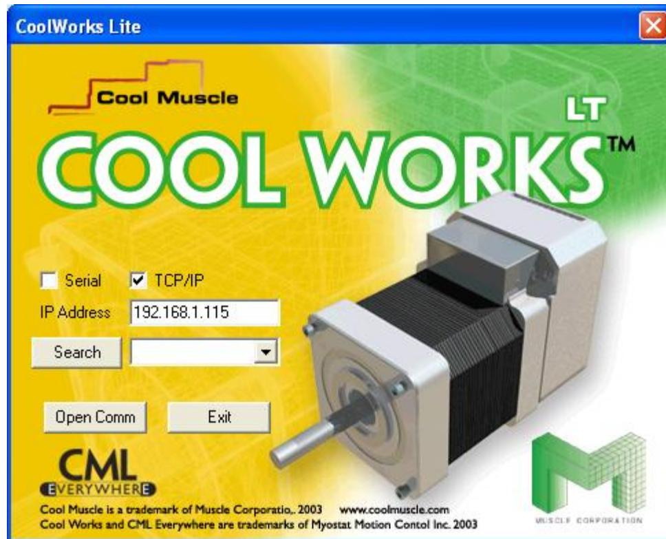
As can be seen in the above screen capture the TCP/IP option is selected and an IP address can be entered. The serial-ethernet bridge uses port 10001 and CWLite automatically sets this.
